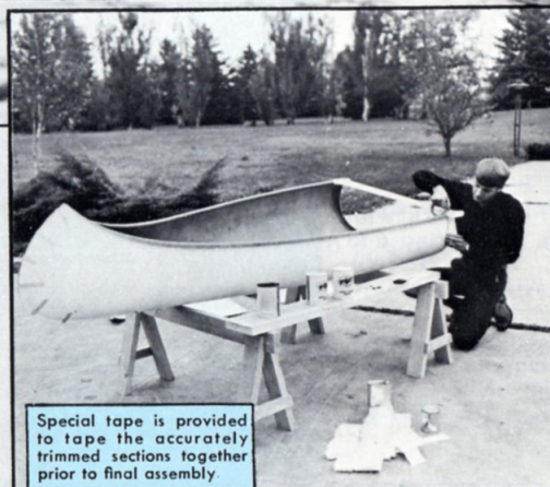
Pre-cut fiberglass mat permanently bonds sections into one piece. Note: Special patented bottom design.
