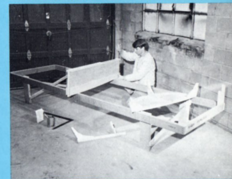
Sub-assemblies such as the transom and centerboard are glued and assembled. Transom is mahogany in keeping with fine boat traditions.
