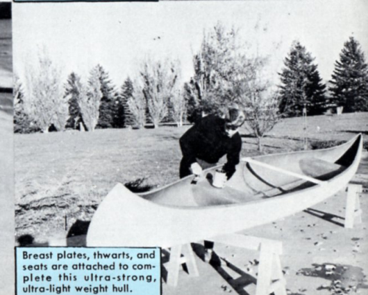
Pre-cut fiberglass mat permanently bonds sections into one piece. Note: Special patented bottom design.
