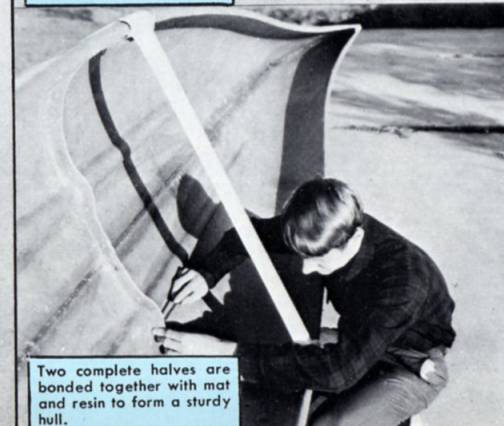
Special tape is provided to tape the accurately trimmed sections together prior to final assembly.
