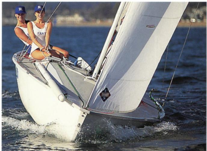
*The Ultimate 20 (above) carves to windward cleanly; a carbon-fiber pole extends to power the asymmetrical chute downwind.*
