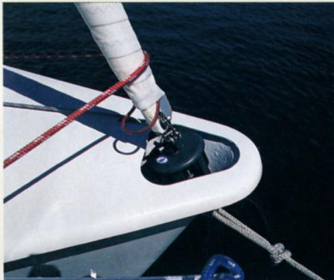
**T**he roller furler, recessed in the bow, is just one of the keep-it-simple details of the 20. Below, the cockpit is clean, simple and comfortable for three crew. Set the 452-square-foot asymmetrical spinnaker, right, and the 20 takes off in true sport boat style.
