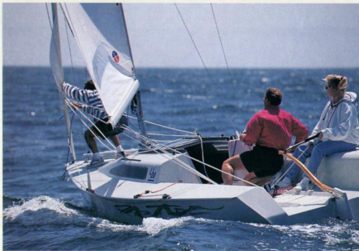
**W**ithout a backstay, the Ultimate 20 is sailed dinghy style—mainsail shape is controlled with mainsheet tension, after giving the rig prebend with the swept-back shrouds before setting sail.
