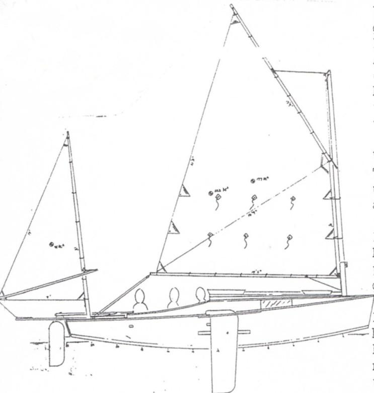
Viola is a fairly large cabin sharpie that uses very conventional glue and nail plywood construction but needs no lofting or building jigs. She is self-righting and self-bailing. I believe a boy could launch and rig her solo in an hour, although practice counts for a lot in operating a boat this large. Actually, when boats get over about 16 feet long, you may not be able to handle them by brute strength in some conditions and you must outsmart them with planning.
