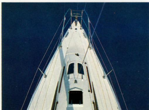
For safety, the deck has molded-in non-skid pattern throughout; upper and lower lifelines surround the deck; and teak handrails run down both sides of the cabin top.
