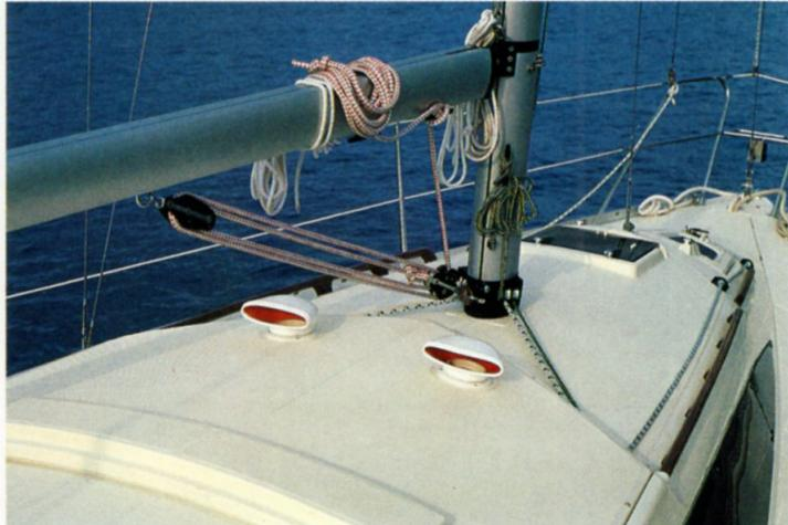
Non-slip patterns are also molded into the cockpit, which is designed so that it is convertible to a "T" configuration for racing. Halyards go beneath the sea-hood and lead to the cockpit where all the winches are located. The YAMAHA-30 can be raced, or just sailed, with a minimum crew.
