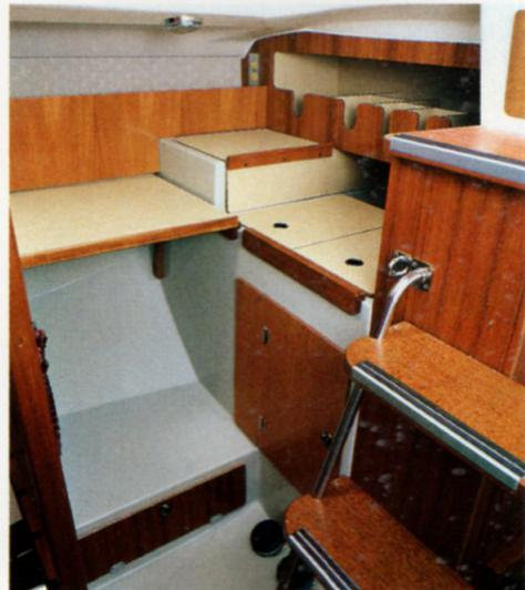
Directly opposite the galley is the navigator's space. A flexible reading light illuminates the big 813mm x 610mm (32" x 24") chart table. Plus, the navigator has his own seat.
