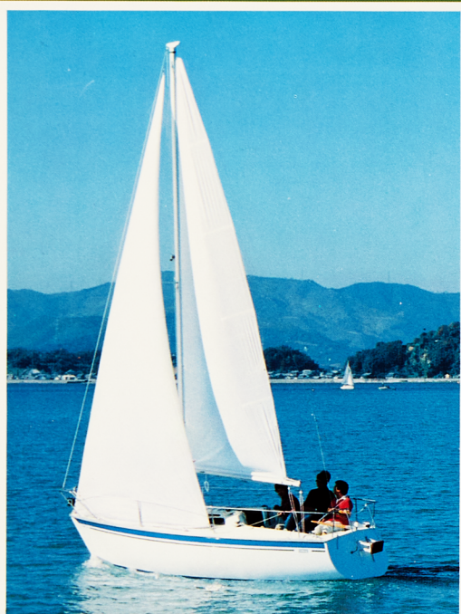
YAMAHA-21JOG L.O.A. .... 20'12" (6.40m) L.W.L. .... 18'3" (5.55m) Beam .... 7'7" (2.30m) Displacement .... 1,100 kg Draft .... 3'11" 4'7" (1.20 1.40m) Ballast .... 450 kg Sail Area .... 195 sq.ft (18.16m 2 )
