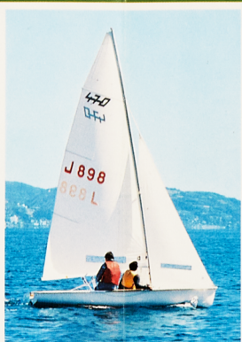
YAMAHA-477 L.O.A. .... 15'5" (4.70m) L.W.L. .... 14'7" (4.44m) Beam .... 5'6" (1.68m) Displacement .... 118 kg Draft C-B up down ... 6" 3'5" (0.15 1.05m) Sail Area .... 137 sq.ft (12.70m 2 )
