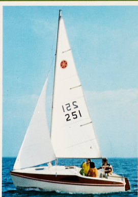
YAMAHA-17 L.O.A. .... 16'8" (4.99m) L.W.L. .... 14'9" (4.50m) Beam .... 6'9" (2.05m) Displacement .... 500 kg Draft C-B up down ... 11" 4'3" (0.55 1.30m) Ballast .... 150 kg Sail Area .... 122 sq.ft (11.30m 2 )
