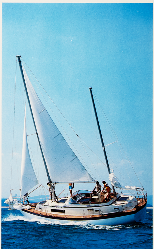
YAMAHA-37CK (Cruising Ketch) L.O.A. .... 36'9" (11.20m) L.W.L. .... 29'6" (9.00m) Beam .... 12'2" (3.70m) Displacement .... 5,420 kg Draft .... 5'3" (1.60m) Ballast .... 2,100 kg Sail Area .... 596 sq.ft (55.40m 2 )
