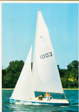
YAMAHA-13 Cicala L.O.A. .... 13'4" (4.07m) L.W.L. .... 12'9" (3.89m) Beam .... 5'5" (1.64m) Displacement .... 112 kg Draft C-B up down ... 6" 3'4" (0.15 1.03m) Sail Area .... 124 sq.ft (11.50m 2 )
