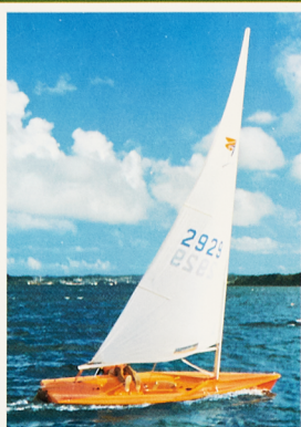
YAMAHA-14 SeaHopper L.O.A. .... 13'11" (4.25m) L.W.L. .... 13'2" (4.02m) Beam .... 4'8" (1.43m) Displacement .... 51 kg Draft C-B up down ... 4" 2'7" (0.10 0.80m) Sail Area .... 83 sq.ft (7.70m 2 )
