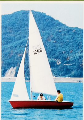
YAMAHA-16 Sealark L.O.A. .... 16'3" (4.95m) L.W.L. .... 15'1" (4.61m) Beam .... 5'11" (1.79m) Displacement .... 150 kg Draft C-B up down ... 6" 3'5" (0.10 1.05m) Sail Area .... 135 sq.ft (12.50m 2 )
