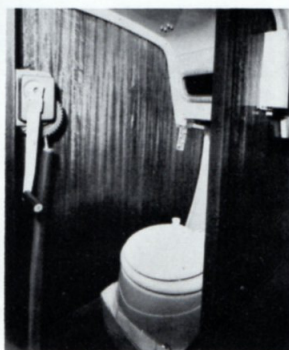
Centerboard winch with removable handle mounted on enclosed head bulkhead out of the way yet readily accessible.
