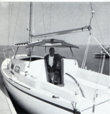
Lifting the "pop-top" provides full 6'2" headroom. Optional acrilan side curtains shown make a comfortable, roomy cabin in all weather.
