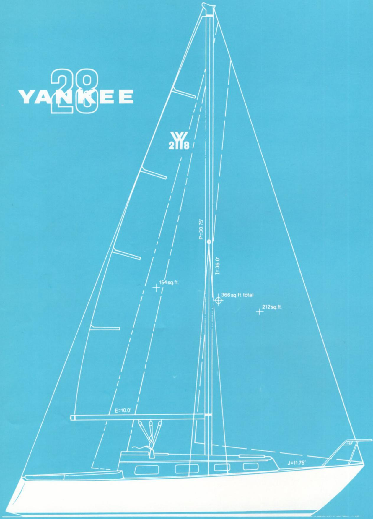
Sail Area 366 sq. ft. • Displacement 6500 lbs. • Ballast 2750 lbs. • L.O.A. 27'9" • L.W.L. 21'10 1/2" • Beam 8'6 3/8" • Draft 4'8"
